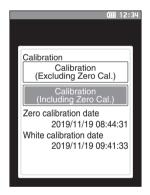
2 Use [▲] or [▼] to move the cursor to "Calibration (Excluding Zero Cal.)", and then press the [Confirmation] key.
