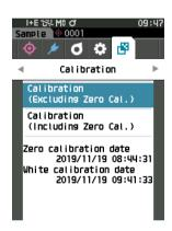
3 Set the instrument in the calibration stage in order to measure the calibration stage's white calibration plate.
