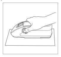
To measure concave surfaces, as shown in the following figure, use the standard accessory flat type battery cover (CM-A218).
